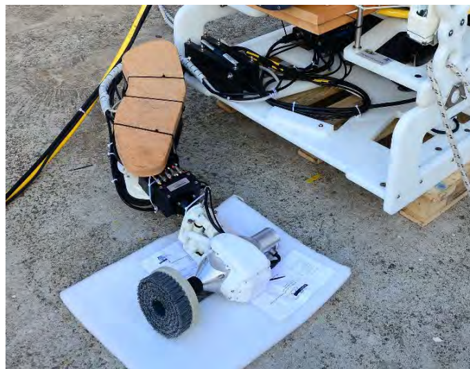
Fig. 2. The re-engineered underwater arm mounted on the skid of the ROV.
