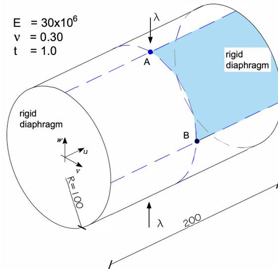
Figure 7: Pinched cylinder: geometry
