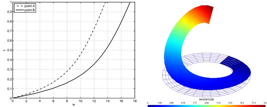
Figure 6: Slit annular plate: equilibrium path and deformed configuration at the last evaluated equilibrium point
