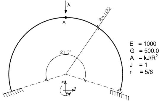
Figure 1: Clamped-hinged arc: geometry
