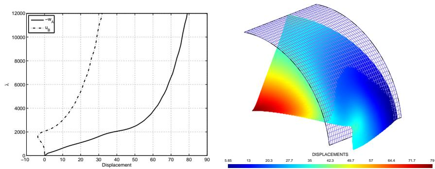
Figure 8: Pinched cylinder: equilibrium path and deformed configuration at the last evaluated equilibrium point
