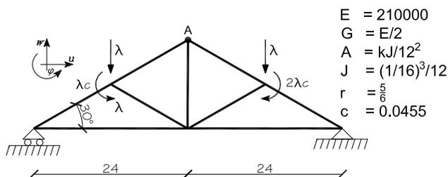
Figure 3: Rigidly jointed truss: geometry
