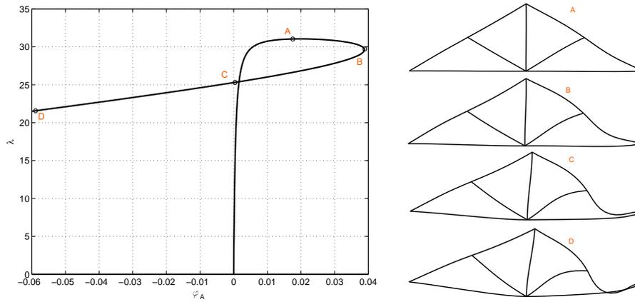
Figure 4: Rigidly jointed truss: equilibrium path and deformed configuration evolution
