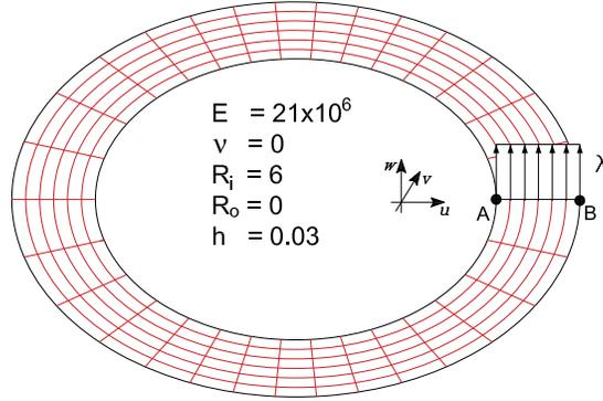
Figure 5: Slit annular plate: geometry
