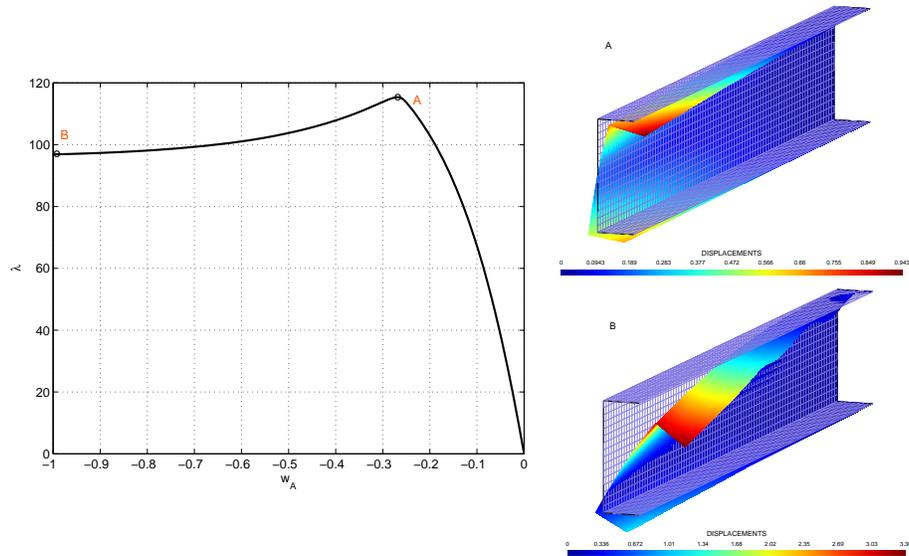
Figure 10: Cantilever beam: equilibrium path and deformed configuration at the last evaluated equilibrium point
