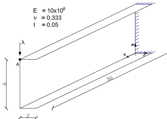
Figure 9: Thin walled cantilever beam: geometry
