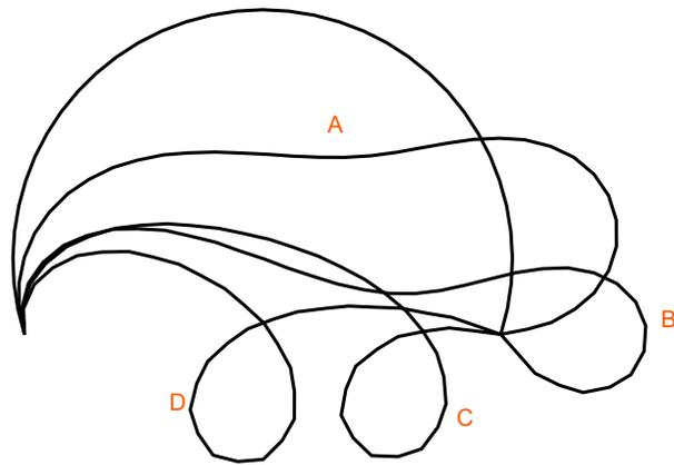
Figure 2: Clamped-hinged arc: equilibrium path and deformed configuration evolution
