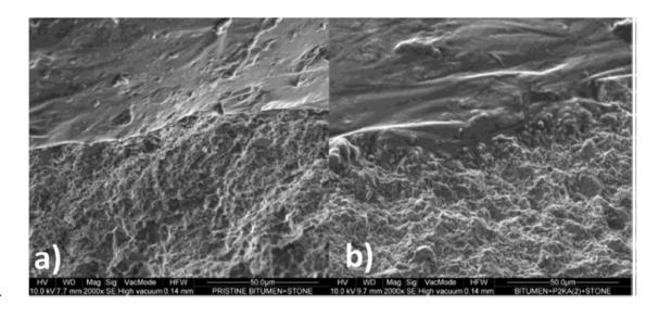
**Figure 4.** SEM images showing a) the interface between pristine bitumen and stone and b) modified bitumen (**B\_0.1%\_P2KA®**) and stone.
