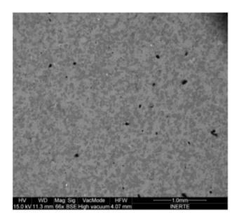
**Figure 3.** SEM image of the inert stone with darker acid silica regions and light basic limestone regions.
