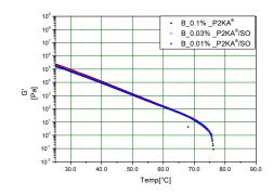
Figure 1. Temperature ramp test (1 Hz) for the modified bitumens'.
