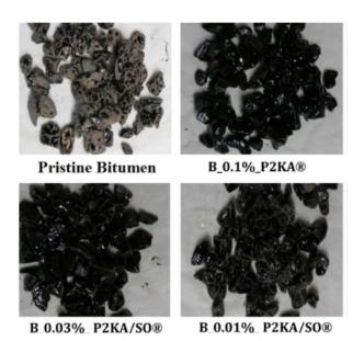
Figure 2. Visual estimation of aggregate surface area covered with bitumen. The images of pristine bitumen and **B\_0.1%\_P2KA®** were taken from reference [3].
