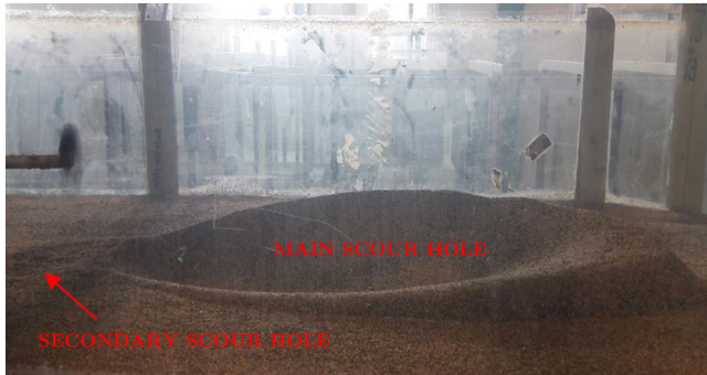
FIG. 1. Photograph of an equilibrium scour produced by a propeller in a laboratory flume.
