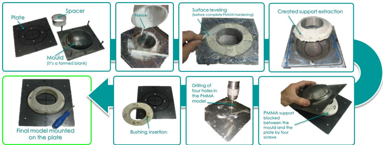
Figure 7. Procedure of support manufacturing.
