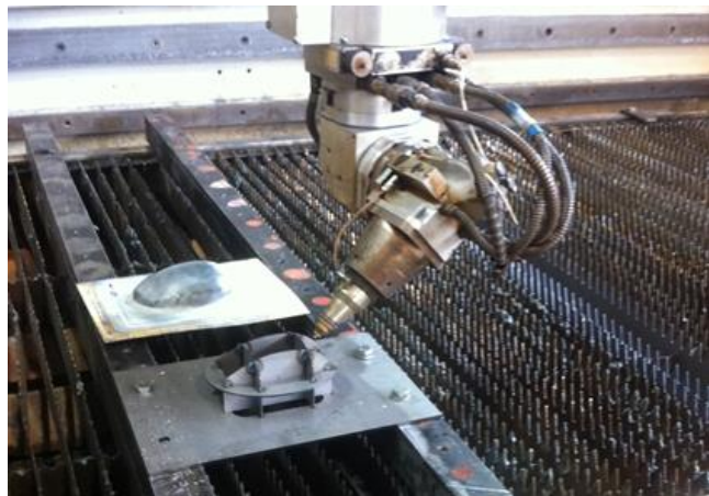
Figure 6. Formed blank positioning for the 3D laser cutting of SPFed and SPIFed parts.
