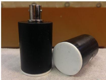
Fig. 4. A picture of the employed broad-band piezo-composite transducers.
