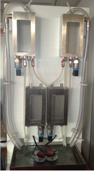
Fig. 10. The laboratory four tanks process.
