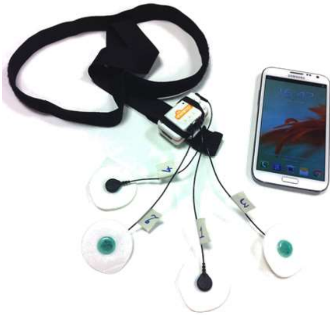
Fig. 9. Wearable 4 leads ECG sensor (using Shimmer2R node) and the smartphone used to collect data.
