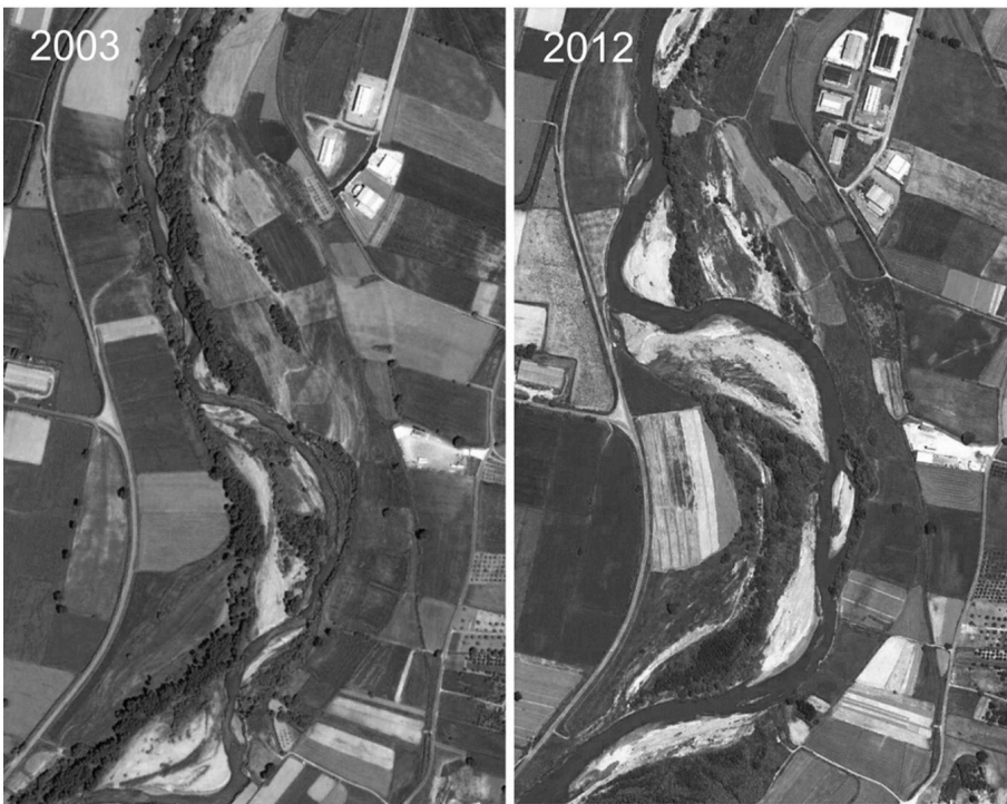
Fig. 6. Comparison of a portion of the Crati reach Cr5 showing consistent channel widening from 2003 (A) to 2012 (B).
